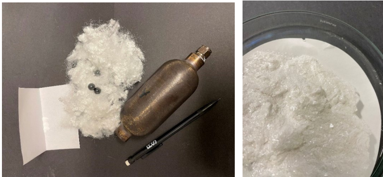
Polyester fibres, as well as lab reactor, catalyst powder, and ceramic balls used for blending (L); Dry BHET monomer (R).
