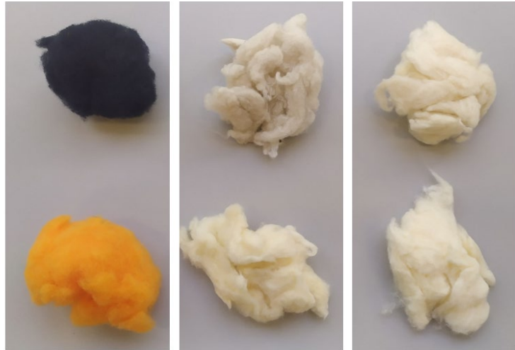
Cotton fibre samples before and after first and second steps of colour removal process.
