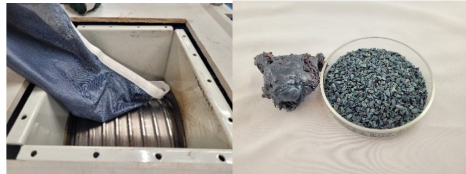
The original technical textile product going into MODIX, and compacted (=melted) polyester lump and the material after grinding.
